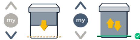
Motor jogs to confirm lower limit
