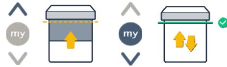
Motor jogs to confirm upper limit
